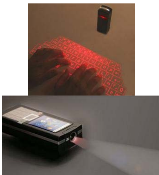
Figure 17. Keyboard and screen projection with mobile phones [2]
